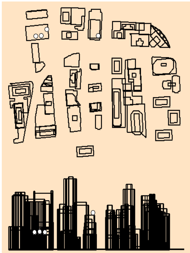
Fig. 4. Outdoor case: The top and elevation view of Rosslyn, VA where we use a (4, 4)-MEA at both the transmitter and the receiver to obtain initial capacity estimates for outdoor wireless loops operating at 1.9 GHz.
