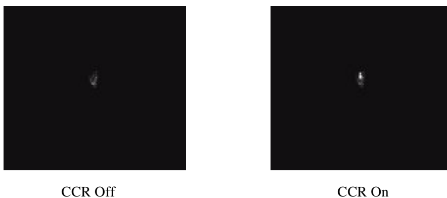
Fig. 45. Images captured by a video camera of the light reflected from a CCR in its off and on states.
