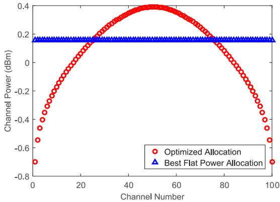
Fig. 4. Optimized power allocation for maximum margin with a homogeneous modulation format and flat amplifier noise. Simulation parameters are as in Fig. 2.
