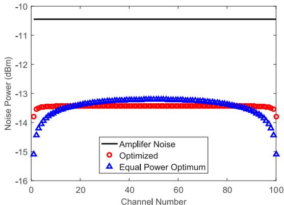
Fig. 3. Amplifier and Gaussian nonlinear noise levels for capacity-maximizing power allocation. Simulation parameters are as in Fig. 2.
