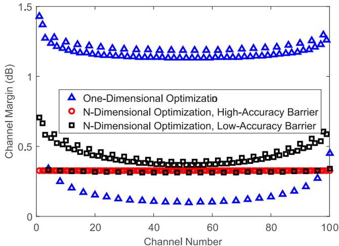
Fig. 7. Channel margins with inhomogeneous required SNRs under various optimization scenarios. Power optimization sacrifices margin in channels with higher margin to maximize the minimum-margin channels resulting in equal margin in all channels. Simulation parameters are as in Fig. 2.
