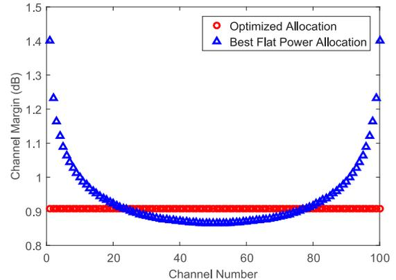
Fig. 5. Channel margins with optimized power allocation for a homogeneous modulation format and flat amplifier noise. Simulation parameters are as in Fig. 2.
