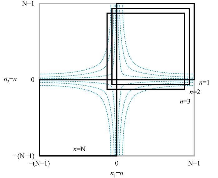
Fig. 1. The  $N \times N$  coefficient matrices for each channel described by equation (3) are sub-matrices of a  $(2N - 1) \times (2N - 1)$  matrix.
