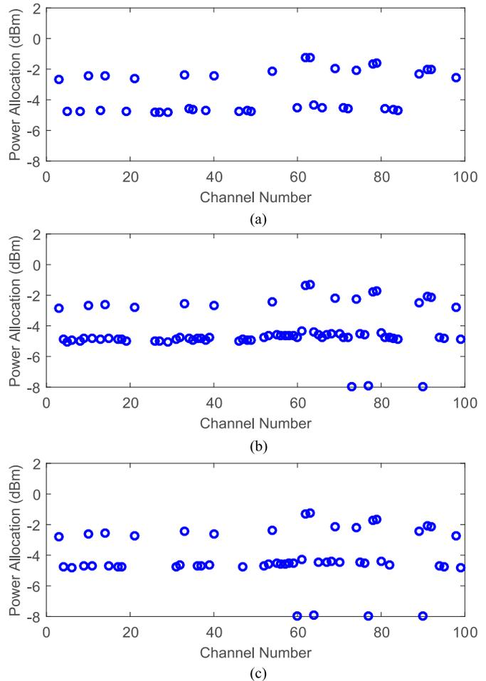
Fig. 9. Margin-maximizing power allocations for randomly assigned paths in three-section mesh network. (a) Section I. (b) Section II. (c) Section III. The mesh network uses 10 spans per section. Other parameters are as in Fig. 2.
