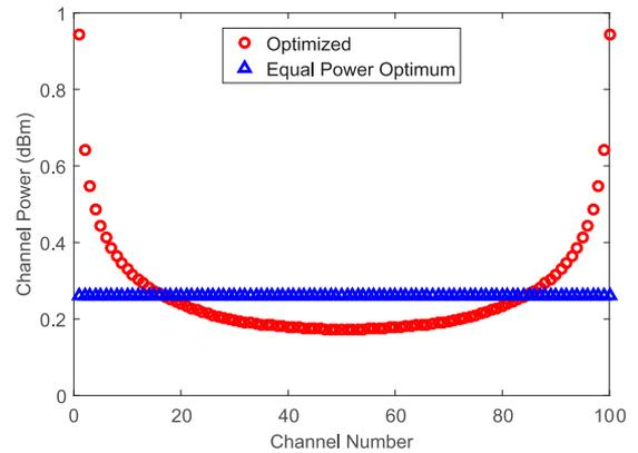
Fig. 2. Capacity-maximizing power allocation and best flat allocation. Simulations consider 40 spans of standard single-mode fiber, each 100 km long, with loss  $\alpha = 0.21$  dB/km, dispersion  $D = 17$  ps  $\cdot$  nm<sup>-1</sup> km<sup>-1</sup>, nonlinear coefficient  $\gamma = 1.4$  W<sup>-1</sup> m<sup>-1</sup>, amplification with flat 4.5-dB noise figure and gain just compensating fiber loss, and a coding gap  $\Gamma = 0.794$  (-1 dB).
