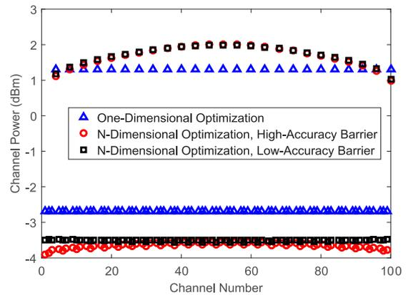
Fig. 6. Power allocation for inhomogeneous required SNRs under various optimization scenarios. Minimum margin optimization with  $N$  dimensions assigns higher powers for channels with high SNR requirements and lower powers for channels with lower SNR requirements than a one-dimensional optimization. Simulation parameters are as in Fig. 2.
