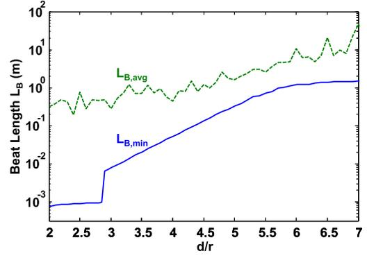
Fig. 2. Minimum (solid line) and average (dashed line) intermodal beat lengths vs.  $d/r$  for seven-core fiber, assuming same parameters as Fig. 1 and  $r = 6.36 \mu\text{m}$ .
