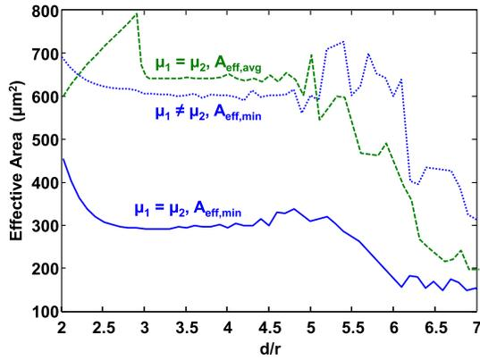
Fig. 5. Minimum intramodal (solid line), minimum intermodal (dotted line) and average intramodal (dashed line) effective areas vs.  $d/r$  for seven-core fiber, assuming same parameters as Fig. 2.
