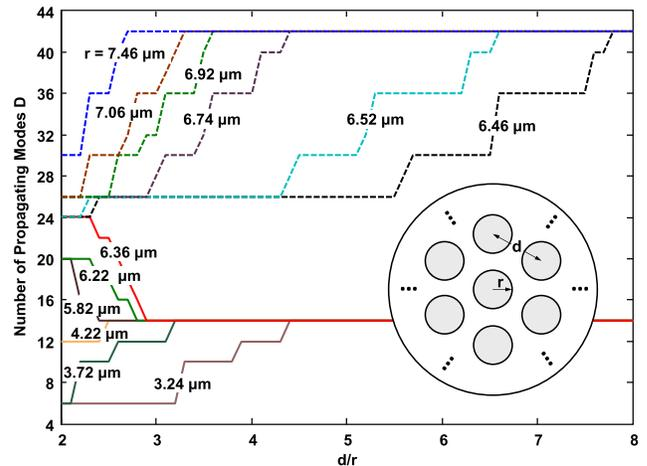
Fig. 1. Number of propagating modes in two polarizations  $D$  vs.  $d/r$  for step-index seven-core fiber assuming  $n_{core} = 1.451$ ,  $n_{clad} = 1.448$  and  $\lambda = 1550$  nm. Inset: fiber with cores of radius  $r$  on hexagonal lattice with spacing  $d$ .
