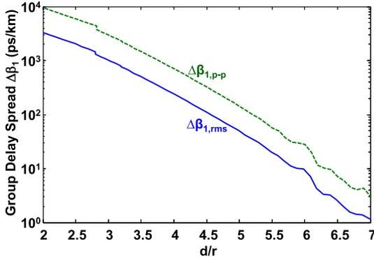
Fig. 3. Peak-to-peak (dashed line) and rms (solid line) GD spreads per unit length vs.  $d/r$  for seven-core fiber, assuming same parameters as Fig. 2.
