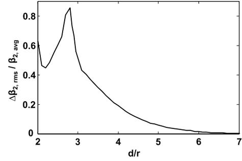
Fig. 4. Rms mode-dependent CD, normalized by mode-averaged CD, vs.  $d/r$  for seven-core fiber, assuming same parameters as Fig. 2.
