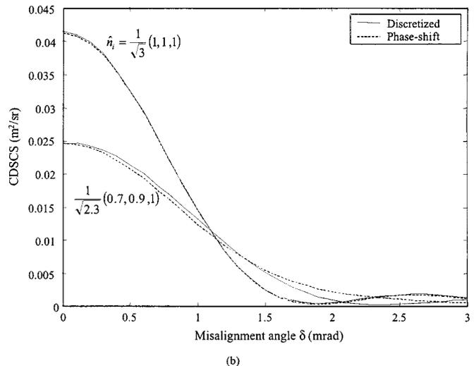
Fig. 6. (a) Misalignment of one of the CCR mirrors by an angle  $\delta$ . (b) CDSCS versus the misalignment angle  $\delta$  computed using both discretized analysis and the phase-shift model. Each CCR mirror is  $250 \mu\text{m}$  square, and the incident directions  $\hat{n}_i$  are  $1/\sqrt{3}(1, 1, 1)$  and  $1/\sqrt{2.3}(0.7, 0.9, 1)$ , respectively.
