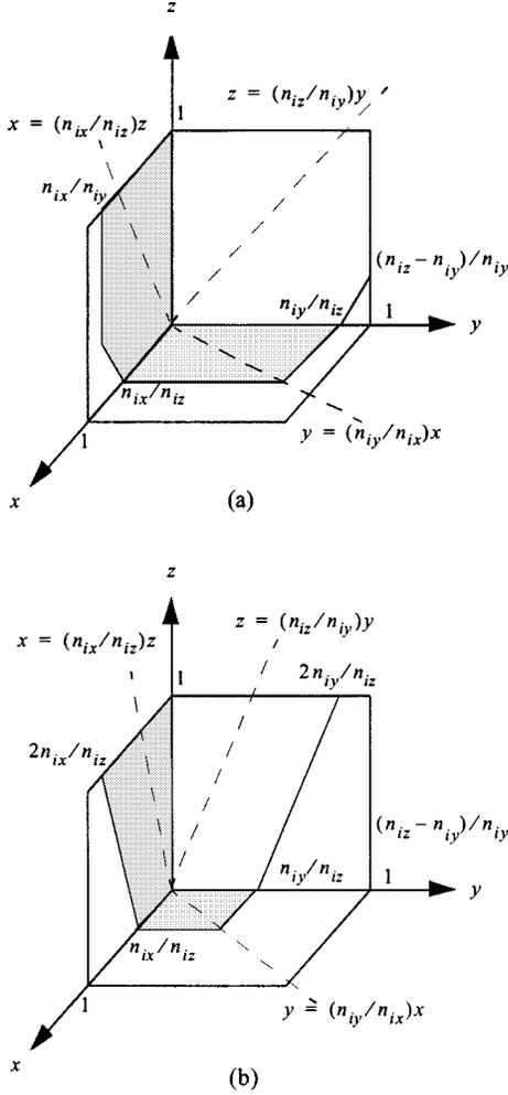
Fig. 2. Effective areas of CCR surfaces with incident direction  $-\hat{n}_i$ , where  $\hat{n}_i = n_{ix}\hat{x} + n_{iy}\hat{y} + n_{iz}\hat{z}$  and  $n_{iz} \geq n_{iy} \geq n_{ix}$ . The two different cases are: (a)  $2n_{iz} \geq n_{iz} \geq n_{iy} \geq n_{ix}$  and (b)  $n_{iz} \geq 2n_{iy} \geq 2n_{ix}$ .
