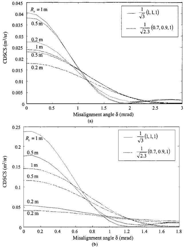
Fig. 8. CDSCS versus the misalignment angle  $\delta$  [as defined in Fig. 6(a)] for different CCR mirror radii of curvature computed by the phase-shift model. The CCR mirror sizes are: (a) 250 and (b) 400  $\mu\text{m}$ . All three mirrors have radii of curvature  $R_c$ , where  $R_c$  takes on the values 1, 0.5, and 0.2 m respectively. The incident directions  $\hat{n}_i$  are  $1/\sqrt{3}(1, 1, 1)$  (solid line) and  $1/\sqrt{2.3}(0.7, 0.9, 1)$  (dashed line), respectively.
