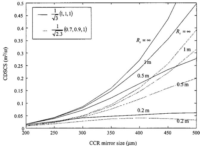
Fig. 7. CDSCS versus the CCR mirror size computed by the phase-shift model. All three mirrors have radii of curvature  $R_c$ , where  $R_c$  takes on the values  $\infty$ , 1, 0.5 and 0.2 m, respectively. The incident directions  $\hat{n}_i$  are  $1/\sqrt{3}(1, 1, 1)$  (solid line) and  $1/\sqrt{2.3}(0.7, 0.9, 1)$  (dashed line), respectively.
