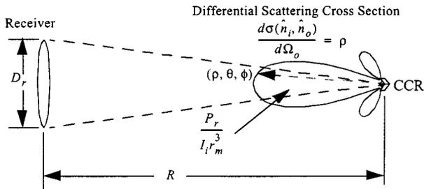
Fig. 4. Calculating the power received by a receiver from a CCR. The DSCS profile is shown in a spherical coordinate system. The angular coordinates  $(\theta, \phi)$  of the spherical coordinate represents the direction of  $\hat{n}_o$ , and the radial coordinate  $\rho$  denotes the DSCS  $d\sigma(\hat{n}_i, \hat{n}_o)/d\Omega_o = \rho$ .
