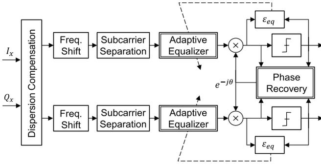
Fig. 5. Detection of two subcarriers per sampling employing adaptive equalization and joint carrier phase recovery (only one polarization is shown). Equalization and phase recovery are done jointly for two polarizations.
