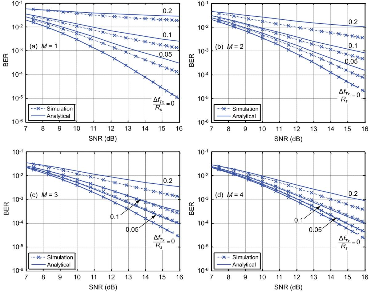
Fig. 8. Average BER versus SNR in the presence of frequency error in transmit lasers of the adjacent subcarriers for simultaneous detection of (a)  $M = 1$ , (b)  $M = 2$ , (c)  $M = 3$ , (d)  $M = 4$  subcarriers. Frequency errors are normalized to the subcarrier spacing. BERs are averaged over a 24-subcarrier superchannel.
