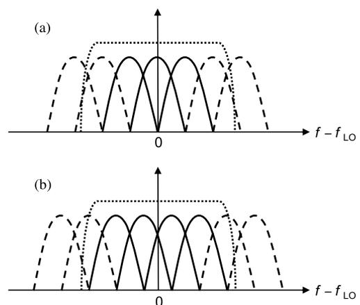
Fig. 4. Frequency spectra for detection of (a)  $M = 3$  and (b)  $M = 4$  subcarriers per sampling for  $R_s = 12.5$  GHz and sampling rate of 75 GHz. The Nyquist bandwidth corresponding to  $|f - f_{LO}| < R_{\text{samp}}/2$  is represented by dotted lines. The central spectral lobes of the desired and interfering subcarriers are represented by solid and dashed lines, respectively.
