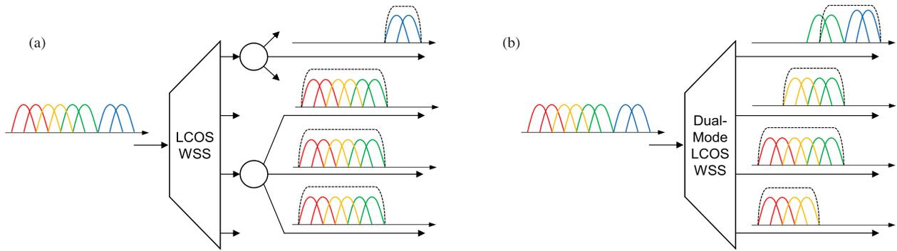
Fig. 3. Possible realizations of colorless gapless demultiplexer at the rightmost node of Fig. 1 using: (a) conventional WSS with star coupler and (b) dual-mode WSS. WSS passbands and central lobes of signal spectra are represented by dashed and solid lines, respectively.
