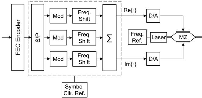
Fig. 2. Block diagram of a transceiver generating  $M = 3$  subcarriers (only one polarization is shown).
