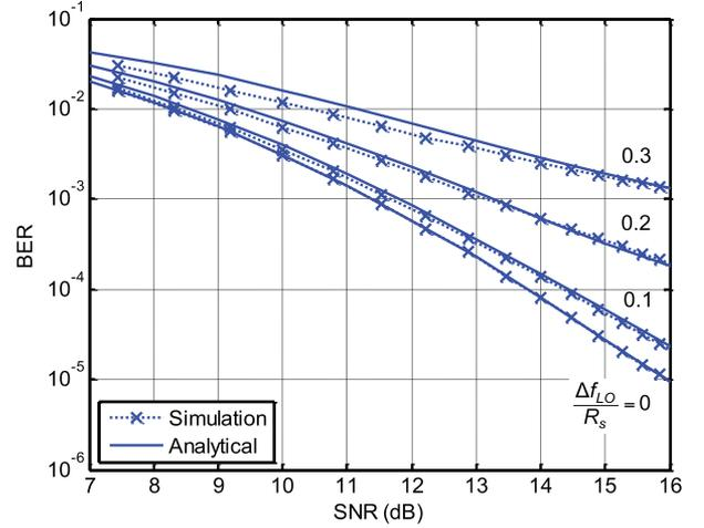
Fig. 7. Average BER versus SNR in the presence of LO frequency-locking error for  $M = 1$ . Frequency errors are normalized to the subcarrier spacing. BERs are averaged over a 24-subcarrier superchannel.
