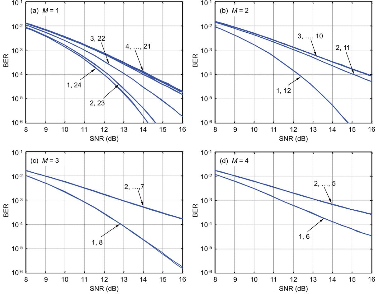
Fig. 6. Average bit-error ratio (BER) versus signal-to-noise ratio (SNR) for each transceiver detecting a 24-subcarrier superchannel. The numbers of subcarriers detected per transceiver are: (a)  $M = 1$ , (b)  $M = 2$ , (c)  $M = 3$ , (d)  $M = 4$ . The transceiver indices are indicated.
