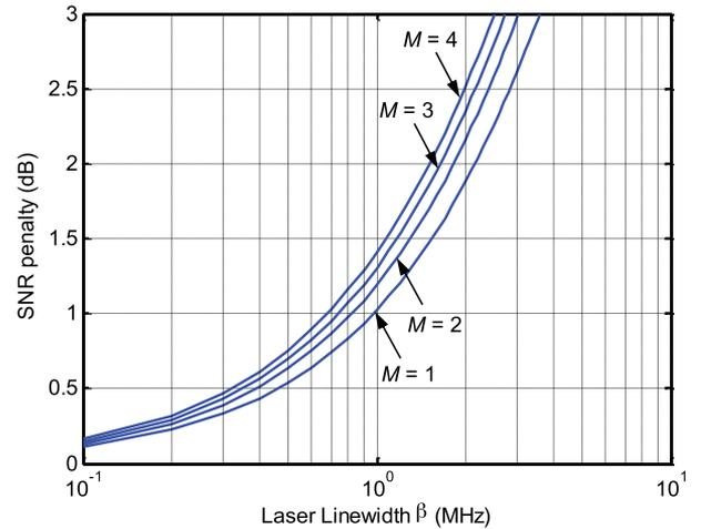
Fig. 10. Worst-case total SNR penalty at  $10^{-3}$  target BER for simultaneous detection of  $M$  subcarriers for  $M = 1, 2, 3, 4$ .
