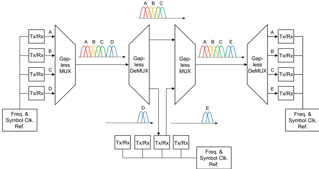
Fig. 1. Optical network with variable-bandwidth superchannels.
