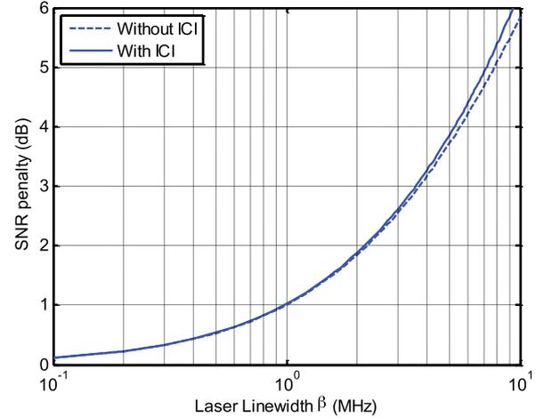
Fig. 9. Worst-case SNR penalty due to phase noise versus laser linewidth for  $M = 1$  at  $10^{-3}$  target BER. The solid and dashed lines show the penalties calculated with and without inter-subcarrier interference.
