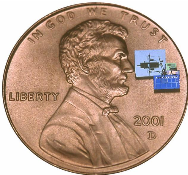
**Figure 2.** Mock-up of the 16mm<sup>3</sup> autonomous solar-powered mote with bi-directional communications and sensing, composed of a 0.25 $\mu$ m CMOS ASIC, solar power array, accelerometer (not yet demonstrated in the system) and CCR, each on a separate die. See Figure 9 for annotations.
