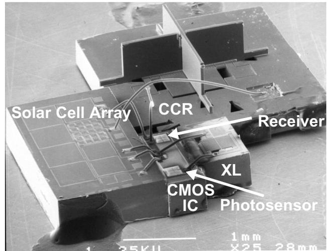
**Figure 9.** Scanning electron micrograph (SEM) of the  $16 \text{ mm}^3$  mock-up shown in Figure 2. The solar cell sizes are adjusted to meet the power requirements of each of the four different sources. The accelerometer is an early version of that described in the text and shown in Figure 4.
