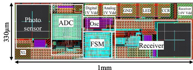
**Figure 8.** Annotated layout of the CMOS ASIC incorporating the oscillator, FSM, receiver, ADC, and photosensor. The pad on the bottom left is the input for the accelerometer or other off-chip sensor. External input voltages applied to this pad have successfully been digitized, but not from the accelerometer.
