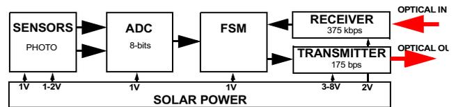
**Figure 3.** High-level functional diagram of the demonstrated mote. The optical downlink and uplink beams are shown separately for clarity, but in practice may be the same beam. (Since the downlink beam is modulated at frequencies well above the uplink signal band, downlink and uplink can share the same channel.)
