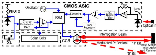
**Figure 7.** Detailed block diagram of the mote. The on-chip oscillator clocks the FSM, which directs the system through a demonstration of all mote functions, including sampling the photosensor and accelerometer, and transmitting both the sensor data and downloaded packets through the CCR. The accelerometer is functional but hasn't been incorporated into the mote yet.
