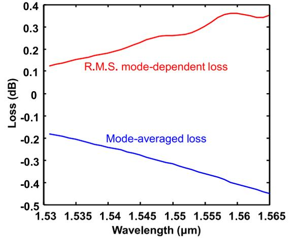
Fig. 5. Mode-averaged and mode-dependent loss of a single LPMFG.
