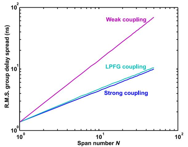
Fig. 6. Group delay spread accumulation in a long-haul MDM system.
