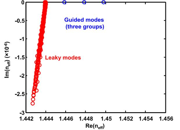
Fig. 2. Propagation constants of leaky and guided modes in GIGDC fiber supporting 12 modes.
