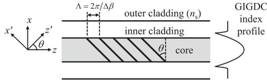
Fig. 1. Diagram of a tilted fiber grating.  $\Lambda$ : grating period,  $\theta$ : grating tilt.
