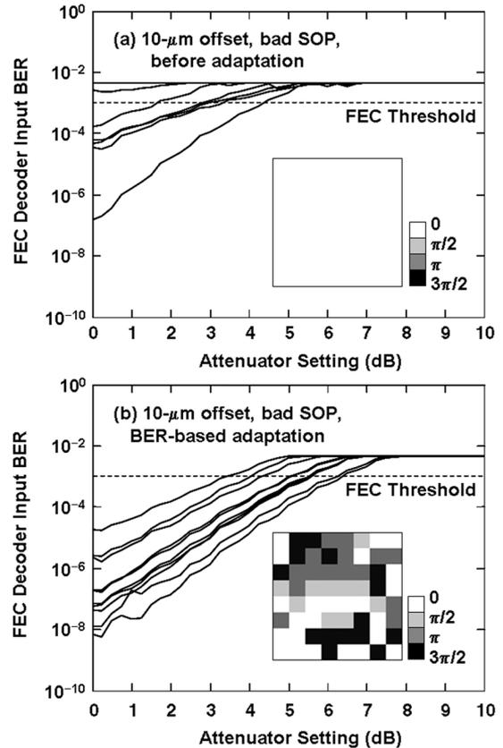
Fig. 4. BERs of the ten data-bearing channels at the FEC decoder inputs, as a function of the transmitter optical attenuator setting, with 10- $\mu$ m offset launch and bad SOP. Insets show the SLM patterns. (a) Before adaptation. (b) After BER-based adaptation.
