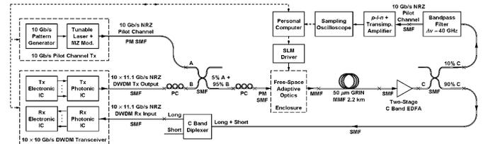
Fig. 1. Experimental setup. PC: polarization controller.
