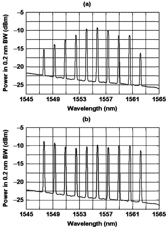
Fig. 3. Optical spectra of the ten data-bearing channels, with 10- $\mu$ m offset launch and bad SOP. (a) Before adaptation. (b) After BER-based adaptation.
