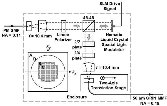
Fig. 2. Free-space adaptive optics subsystem. Inset: SLM in the Fourier plane of the input face of the MMF. A) boundary of SLM active region. B) Block structure of SLM pattern. C) Circle enclosing 95% of power of beam incident on SLM, corresponding to an NA of 0.11 at the MMF input. D) Circle corresponding to the MMF NA of 0.19.
