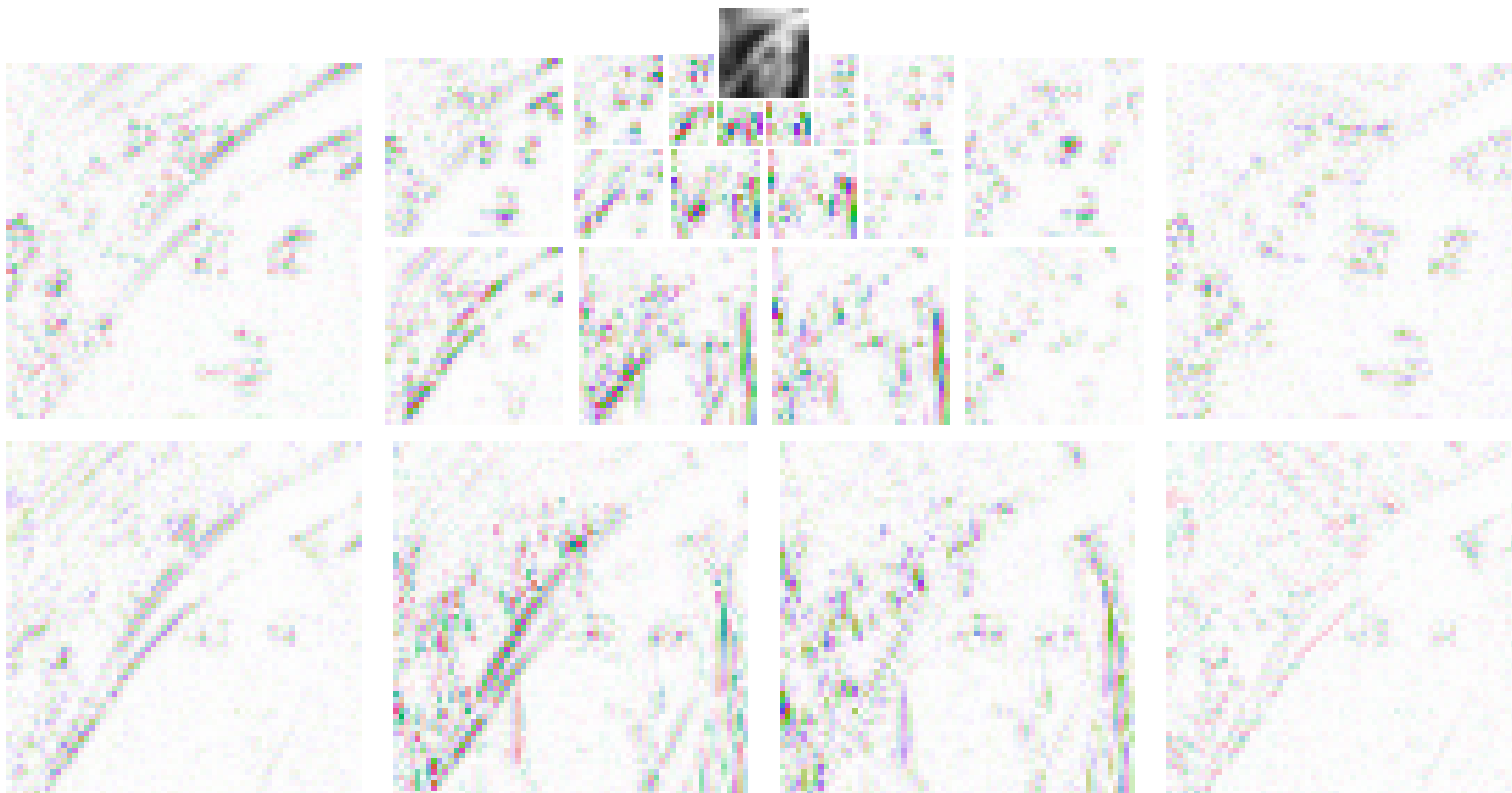
Figure 4: Four-level DT-CWT decomposition of Lenna into 6 subbands per level (only the central 128 \times 128 portion of the image is shown for clarity). A colour-disc palette (see previous slide) is used to display the complex wavelet coefficients.
