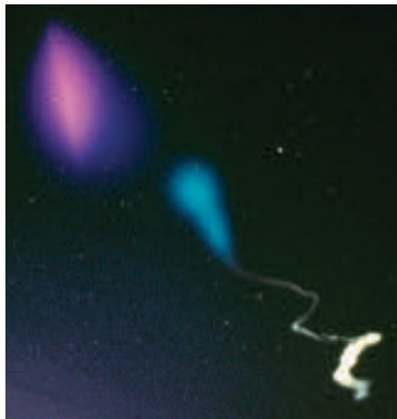
Photograph of a barium ion cloud release (pinkish-reddish color) developing striations along the magnetic field line as a result of the F-layer ionospheric electric field. Also shown in the vicinity of the Ba + cloud is a neutral Ba/Sr cloud. Drifts of these clouds are measured using photographs obtained simultaneously from two camera stations. Also shown is a TMA (trimethyl-aluminum) cloud illustrating the multiple turns of the neutral wind vector between 90 and 140 km. (NASA attribution)
