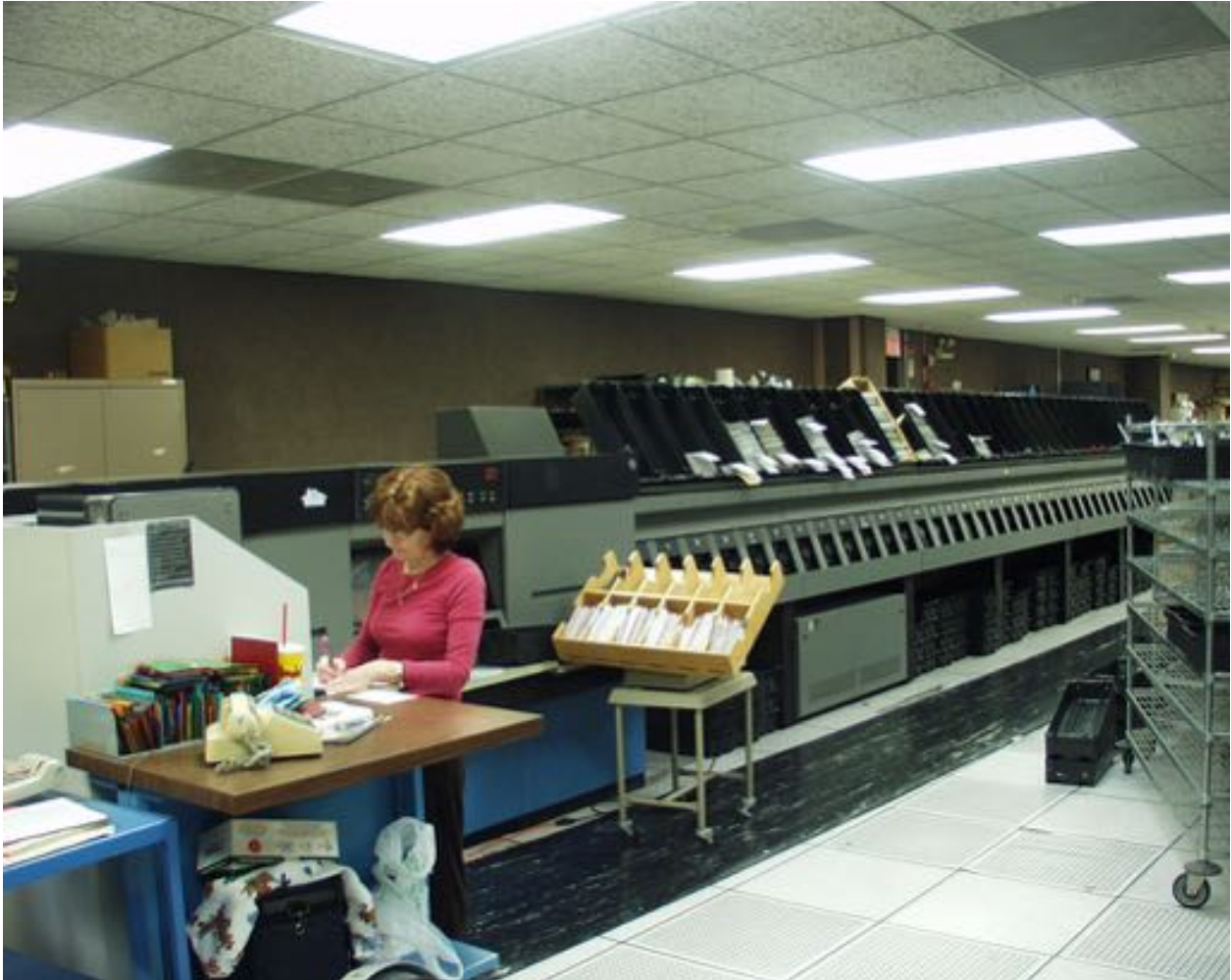
The IBM 3890 check sorter was introduced in 1973 and could process 2400 6" checks per minute. This is a later model than the one I was introduced to in 1968.
