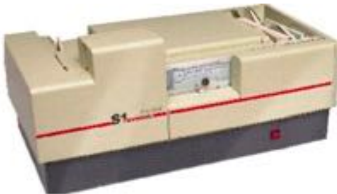
Medium speed check scanner used to create front and back images of checks.
