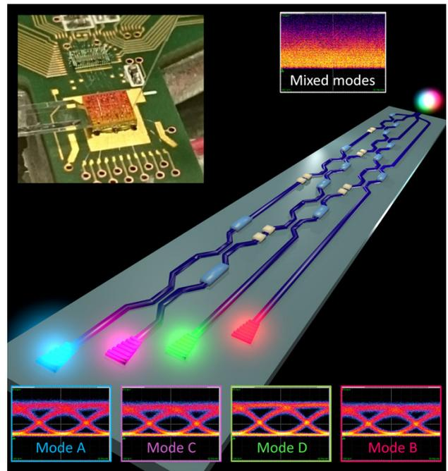
Information encoded in strongly mixed modes (A, B, C, D), sharing the same wavelength and polarization, is recovered by a self-configuring silicon photonics mesh (inset photonic-chip photo), which can automatically reconstruct, separate and sort out the original beams.
