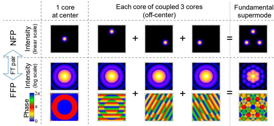
Fig. 1. The relationship between the NFPs and FFPs of a single core and of coupled cores.
