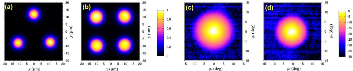
Fig. 2. Two-dimensional (a,b) NFP intensity (linear scale) and (c,d) FFP intensity (decibel scale) images of (a,c) 3CF and (b,d) 4CF.
