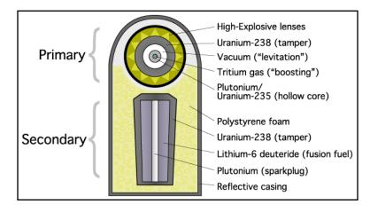
Fission weapons are sometimes called atomic bombs, while fusion weapons are also known as hydrogen bombs or thermonuclear weapons. The basic components of a fusion weapon are shown in this diagram (source: Wikimedia Commons). The "primary" is basically an implosion fission weapon that is used to ignite the
